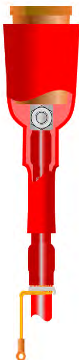
RHSB Straight Heat Shrinkable Boot
